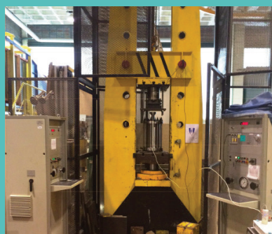
Hgh-pressure triaxial cell, CERENA
